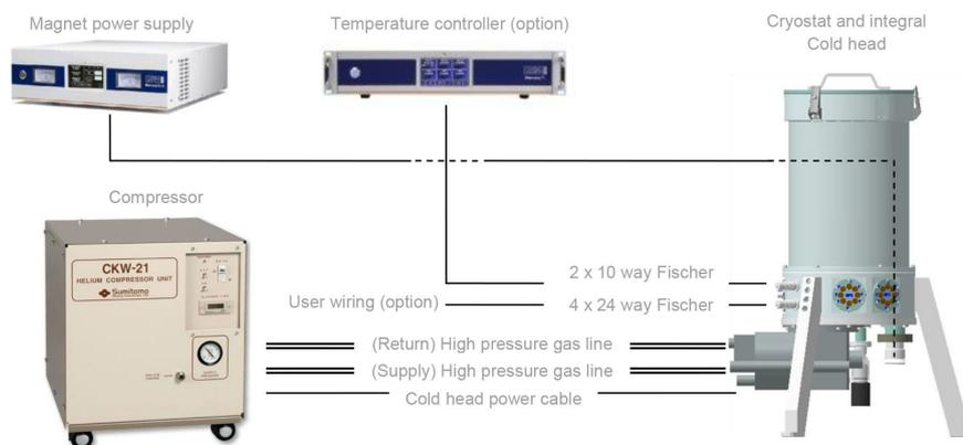
Schematic diagram of Sample Puck Tester system
